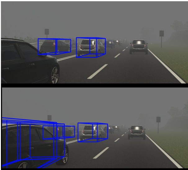
Fig. 3. (Top to bottom) Testing result on foggy dataset using 200 epochs and pretrain models
