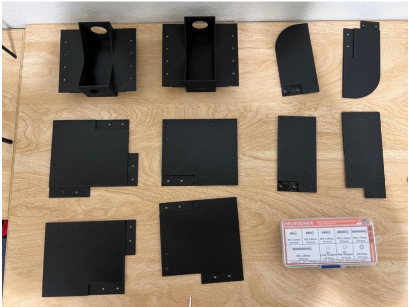
Figure 10. 3D print the chassis as parts.
