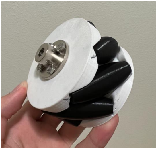
Figure 5. Proper mecanum wheel
