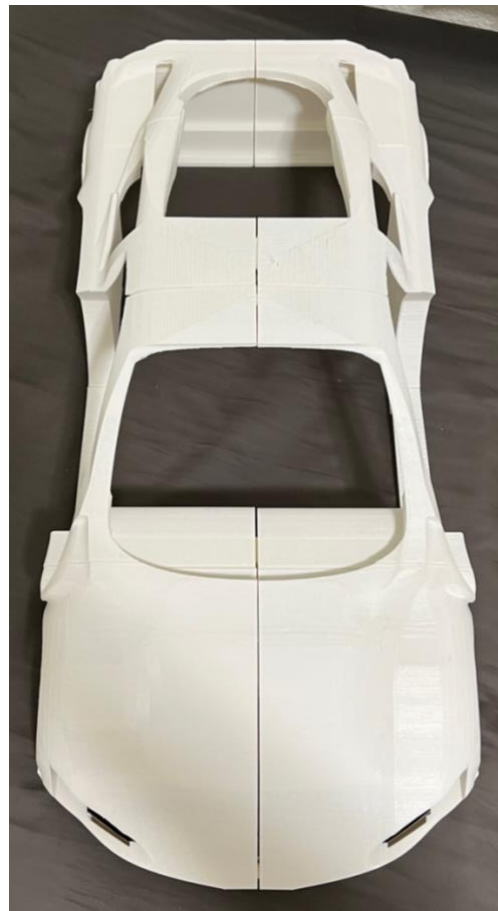
Figure 21-22. Assemble the Tesla Roadster from 3D-printed parts.
